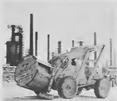
In addition to lifting equipment, this dual-purpose Super 8 High-Lift can also carry material such as this reel of steel cables.
